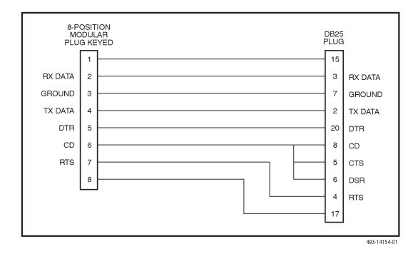
Figure D-6. COM Port-to-Terminal/Printer Cable
